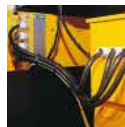
Humidity protection (gland box & special impregnation)
